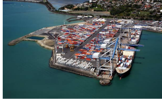
Port of Auckland – land on left side of photo formed by reclaimed dredge material
